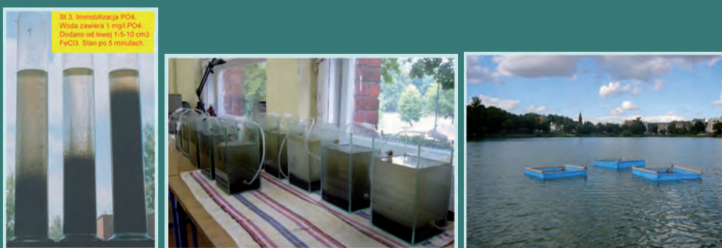
Fig 2 - from the left: - phosphate inactivation with FeCl 3 during sediment resuspension- proper dose. - application of Al 2 (SO 4 ) 3 , FeCl 3 , Phoslock, and FeCl 3 + Ca(NO 3 ) 2 into water, and into sediment. -enclosures in lake Jelonek
