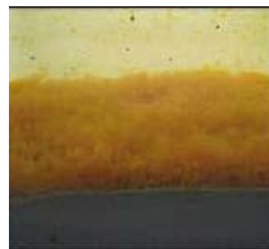
Picture 4 – homogenous layer of a coagulant after it has dropped onto the surface of sediments – laboratory conditions (aquarium 10x10x20 cm), impossible to achieve in a natural water reservoir.
