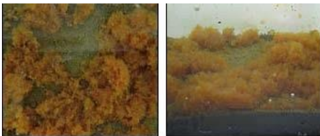
Picture 5. Fractured layer of coagulant due to the above mentioned factors (in the photo on the right you can see gas bubbles coming out of the sediments and fracturing the homogeneity of the coagulant's layer).
