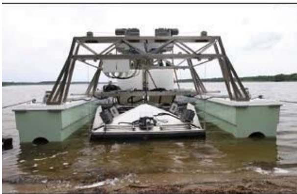
Picture 6. The vessel with an underwater module visible in the dock of the surface module. Due to poor water transparency during reclamation works it is impossible to present photos of the underwater module during application
